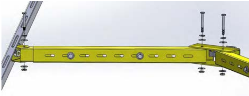
Figure 13. Secure support rails to panel mounting rail and lower bucket bracket
