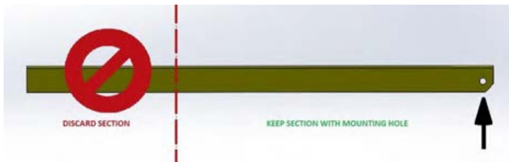
Figure 12. Discard section for larger tilt angles (65° and above)
