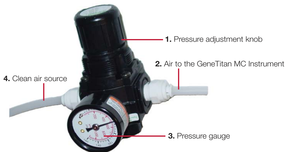
Figure 4 The clean dry air unit
