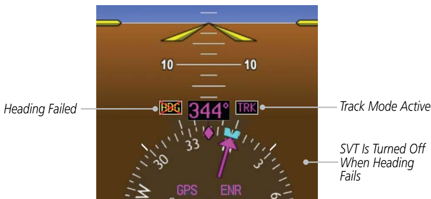
Figure 1-13 Track Mode shown as Active when Heading Info has failed
