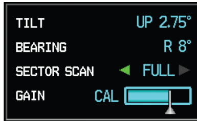
Figure 4-81 Highlight Gain Cal Value
