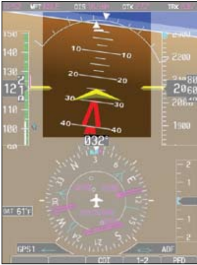
Figure 2-15 Extreme Pitch Indication Nose Down
