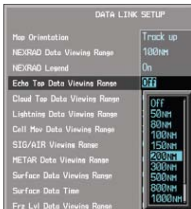
Figure 4-41 Echo Top Viewing Range Selection
