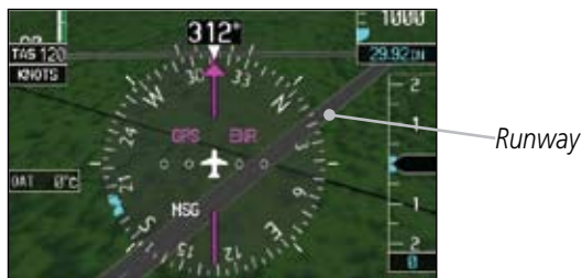
Figure 5-39 Depiction of Runway with a Loaded Flightplan
