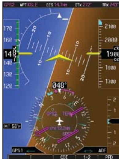
Figure 2-17 Extreme Roll Indication with Display Declutter
