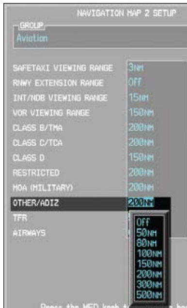
Figure 3-61 Navigation Map Other/ADIZ Viewing Range Selection
