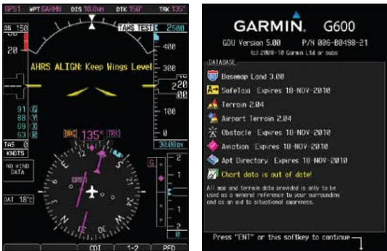
Figure 1-14 System Startup Pages
