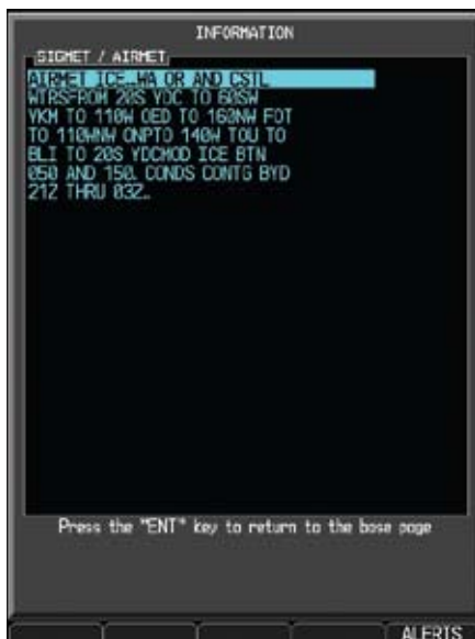
Figure 4-48 XM Weather - AIRMETS
