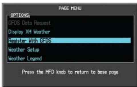
Figure 4-93 Select GFDS Registration
