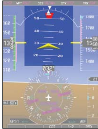
Figure 2-16 Extreme Pitch Indication Nose Up
