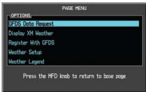
Figure 4-99 Select GFDS Data Request
