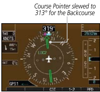
Figure 2-34 Auto-Slewing HSI with Localizer Backcourse Loaded and Shown with the Corresponding Approach Plate
