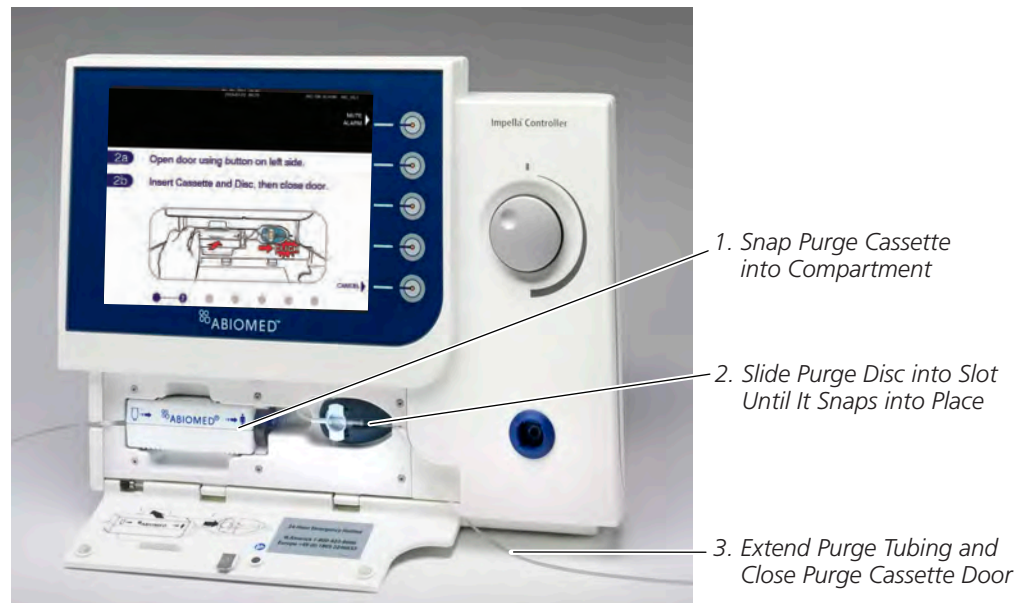
Figure 5.4 Inserting Purge Cassette into Automated Impella® Controller
