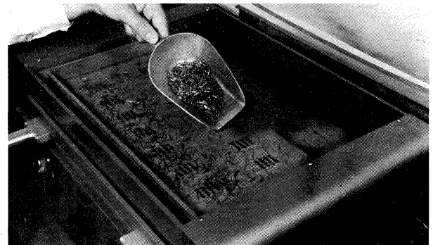
3. Vibrator is turned on and loaded (above) with pins, after a 15 - 30 second cycle 99.9% of the holes have a pin in them (100% fill is common).
