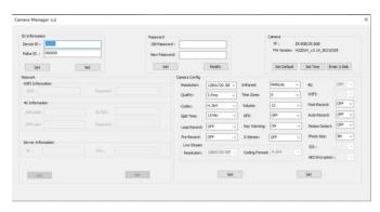
3, Click "Enter U Disk" (upper right corner) to make camera to be recognized by PC as a folder. You can check all files from the camera folder.
