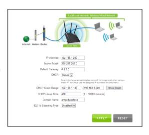
Note: If you choose to use a Static IP address for the Access Point, you will no longer be able to access the web menu using <a href="http://setup.ampedwireless.com">http://setup.ampedwireless.com</a>. You must use the assigned IP address to acces the web menu.
