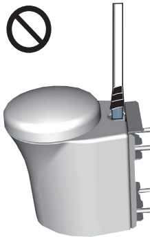
NG: PVC pipe can be seen.
