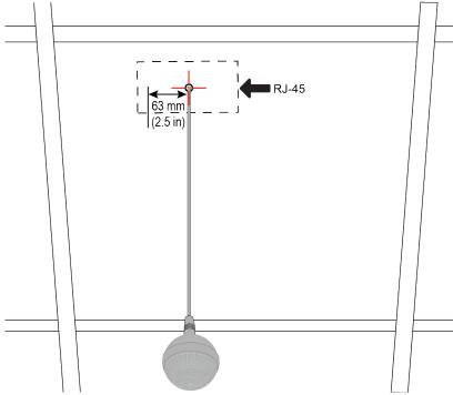
If you can't see the RJ-45 connector, look for the small black button on the microphone cable. Facing that button at the 12 o'clock position, the sensor is located toward the 9 o'clock position.
