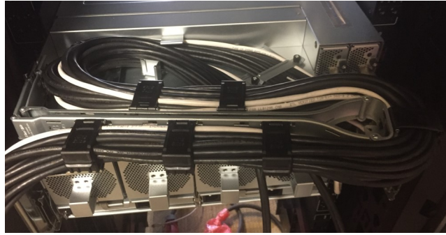
Figure 55 Enclosure Cables routed through CMA
