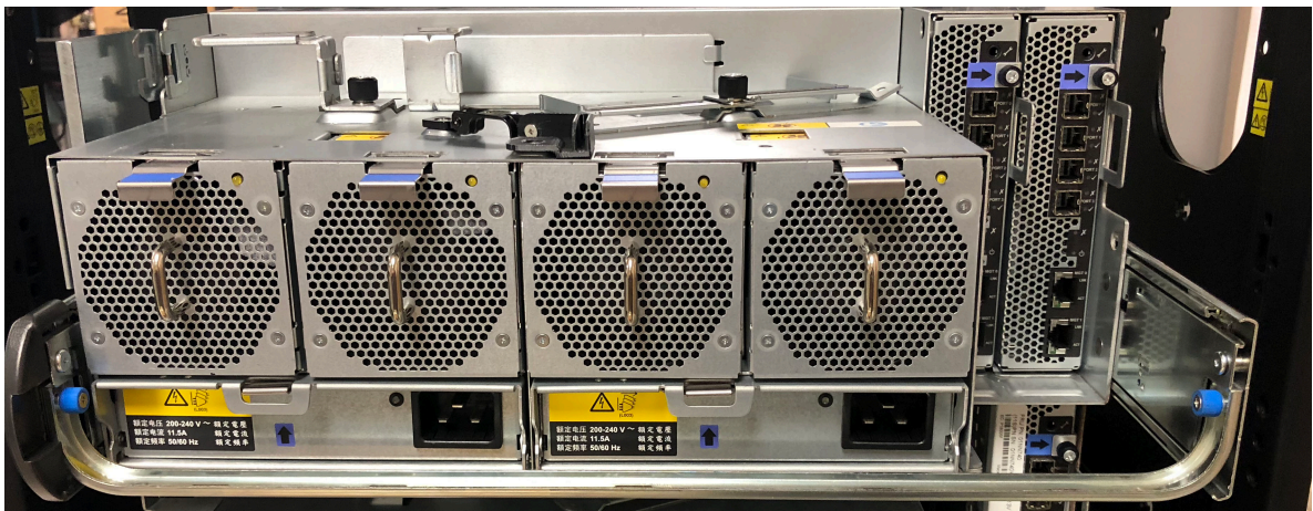
Figure 51 Crossbar installed on the 4U106 enclosure between 2 rails
