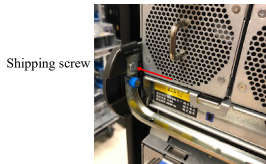
Figure 52 Shipping screw installed
