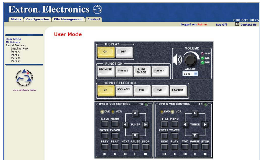
A User Mode default Web page for a System 5 IP (see the note below) that has been configured using Global Configurator
