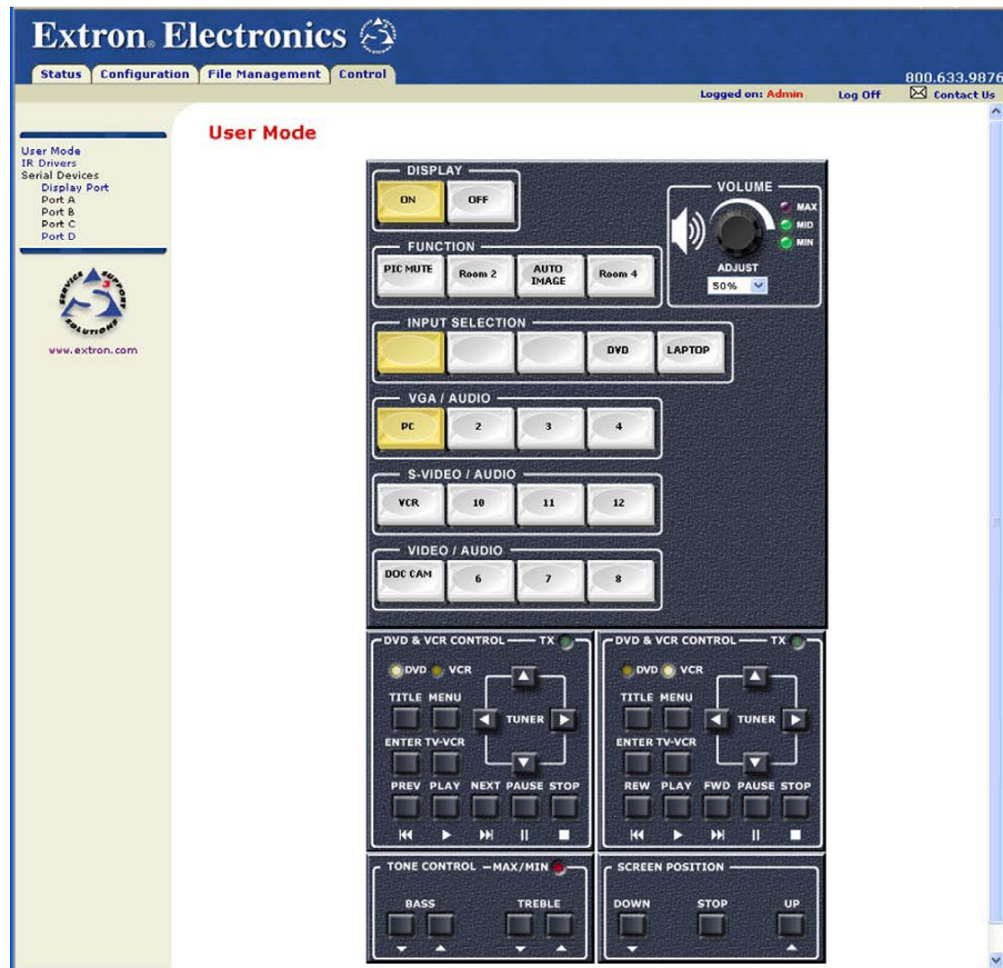
A User Mode Web page for a System 5 IP with an MPS 112 as a secondary switcher
