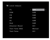
All of the system's speakers will appear with their current level settings. You can adjust each speaker's level between -10 dB and +10 dB in 1 dB increments.
