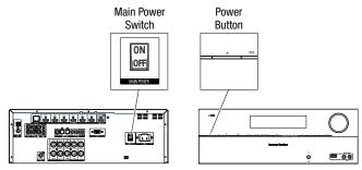
Unless you will not be using the AVR for an extended period of time, leave the Main Power switch set to "On." When the Main Power switch is turned off, any settings you have programmed will be preserved for up to four weeks.
