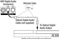
Optical-Equipped Source Device
