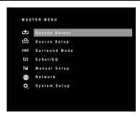
4. Use the remote's arrow and OK buttons to select "Source Setup." If there is a Source Selector for which you want to assign different video or audio connections. use the left/ right arrow buttons to select it, and press the OK button.
