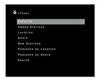
With the vTuner screen (above) displayed, the AVR will automatically connect to the Internet via the www.radioharmankardon.com portal. To select a stream, use the Up/ Down buttons to select a category.
