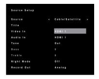
Select "Video In" and use the left/right arrow buttons to select the video input connector you want to assign to the Source Selector button. Press the OK button.
