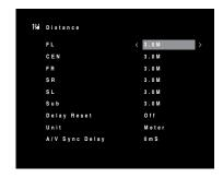
Enter the distance from each speaker to the listening position that you measured in Step Two and recorded in Table A3 in the Appendix (see page 30). Select a speaker, then use the Left/Right buttons to change the measurement. You can enter distances between 0 and 30 feet (9m). The default distance for all speakers is 10 feet (3m).
