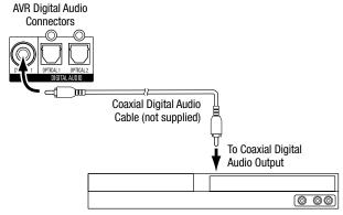
Coaxial-Equipped Source Device
