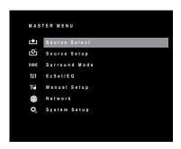
The Master menu consists of seven submenus: Source Select, Source Setup, Surround Mode, EzSet/EQ, Manual Setup, Network and System Setup.
