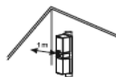
Ⓜ Install the correlation detector at a distance of more than 1 m from the wall
