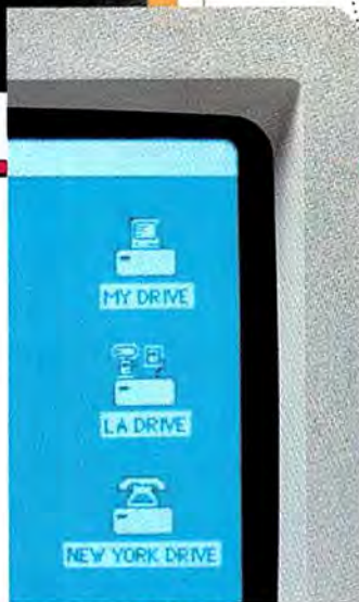
Local or remote hard disks appear on the screen as icons to be opened whenever he wishes.
