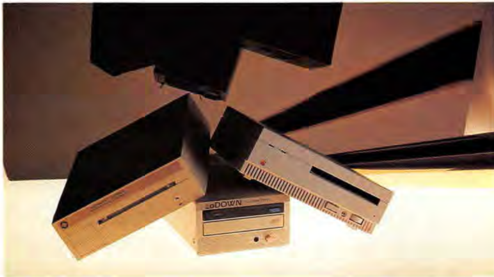
The three drives available for the Macintosh all connect to the SCSI port: (from left) the Laser Magnetic Storage International CM 131, the ALOT (formerly LoDown) CD ROM, and the Apple CD ROM drive.
