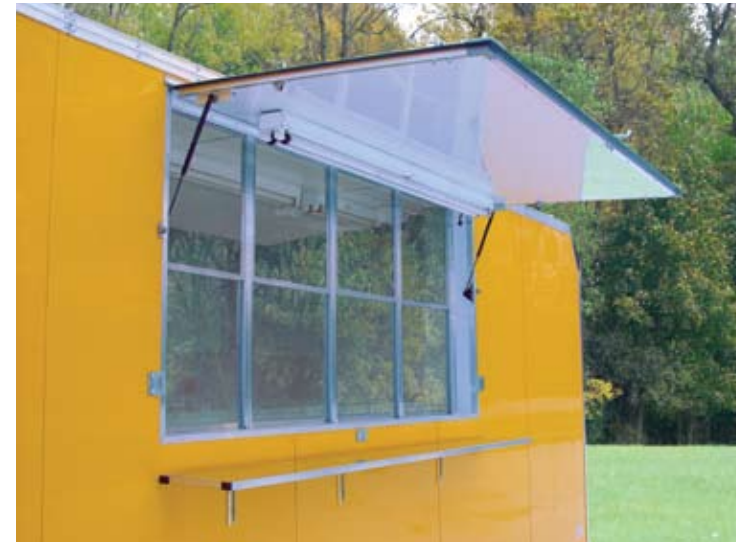
Awning door with fluorescent light and exterior removable shelf under serving window
