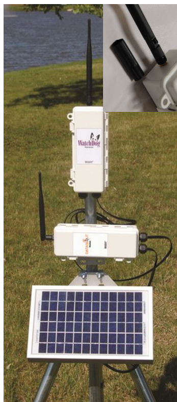
Figure 9. Retriever and DataScout setup with solar panel. Stabilizer shown in inset photo
