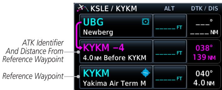
Figure 4-15 ATK Inserted Before Reference Waypoint
