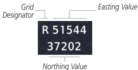
Figure 15-49 Irish National Grid Position Format Detail
