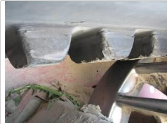
Typical Drive Lug Break-in Wear
