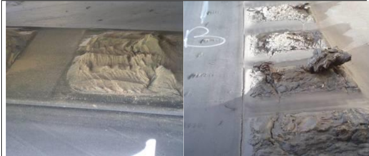
Jagged Separation (Guide Lugs (LH) and Drive Lugs (RH))
