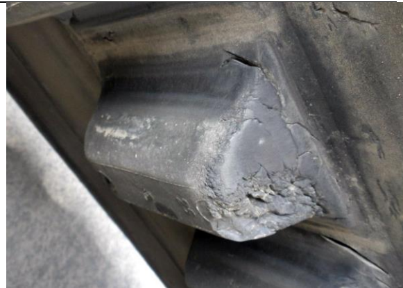
Typical Drive Lug Mid-Life Wear
