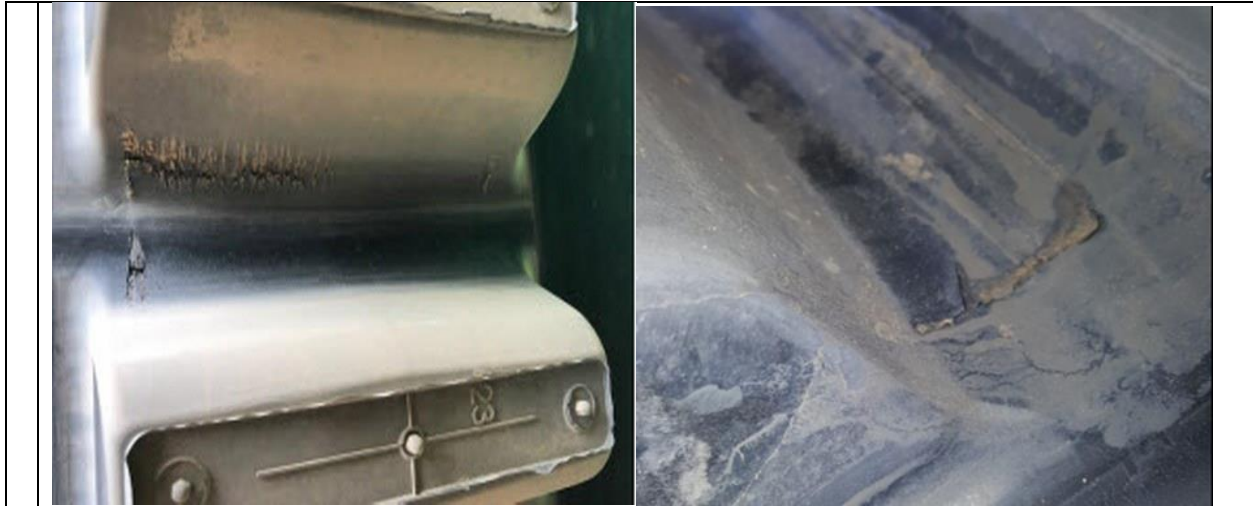
Drive Lug Reinforcement Layer Exposure
