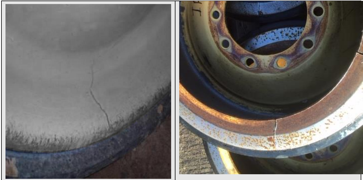
Drive Wheel, Midroller or Idler Cracks
