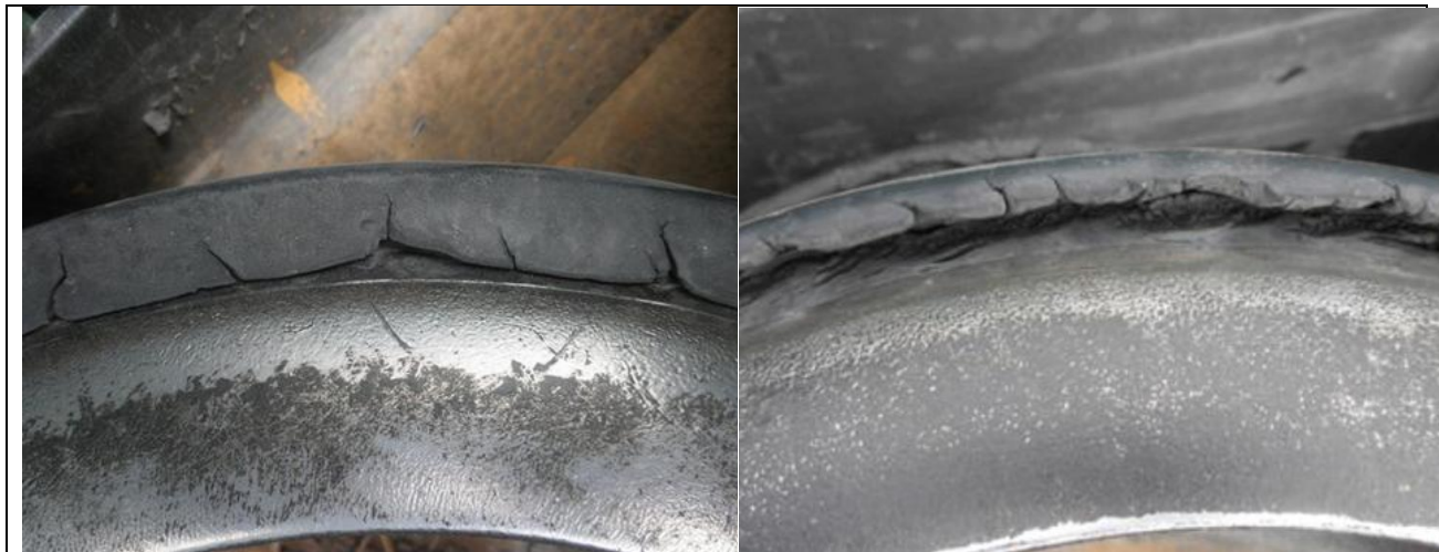
Typical Midroller Edge Wear (Mid life and late life)
