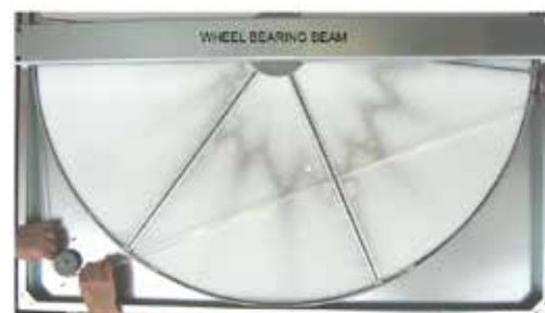
Figure 61: Positioning the Red Belt Retainer and Placing the Belt Over the Pulley (Steps 8 and 9).
