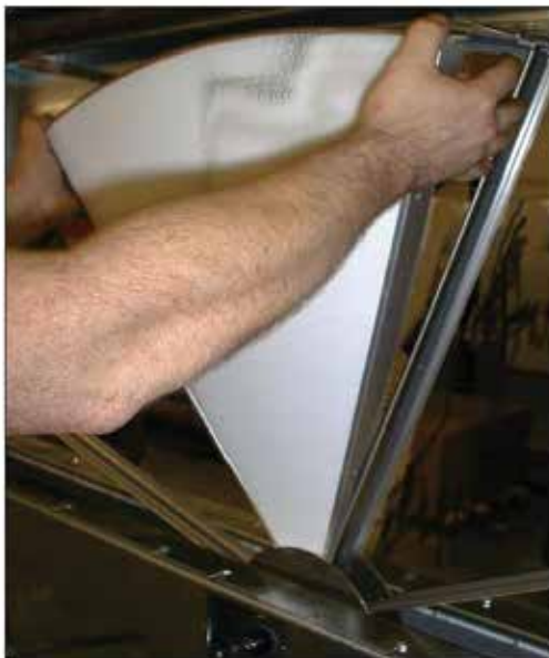
Figure 55: Positioning the Wheel Segment (Step 2).
