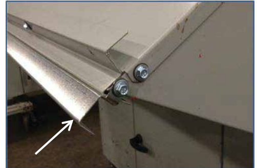
Figure 28: Location of Top Filter Rail (Step 4A).
