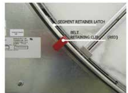
Figure 61: Positioning the Red Belt Retainer and Placing the Belt Over the Pulley (Steps 8 and 9).
