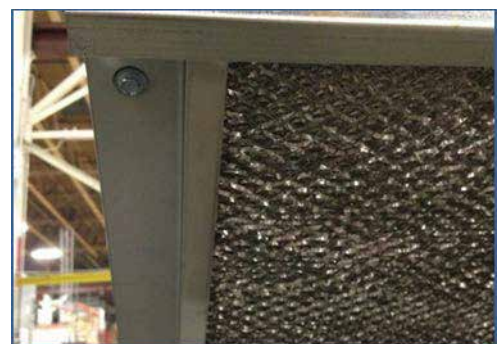
Figure 31: Install Side Spacers (Step 6).
