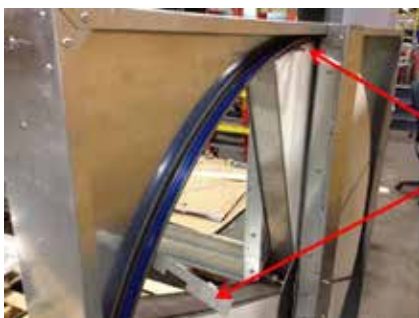
Figure 52: Location of Retainer Clips.
