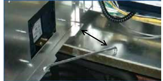
Figure 93: Replacing the Tie-Back Rod into the Door Lip Before Closing the Door.
