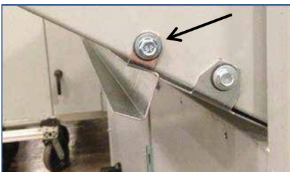
Figure 29: Location of Bottom Filter Rail (Step 4B).
