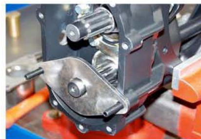
This little tool holds the jackshaft while you tighten and torque the yoke nut.
