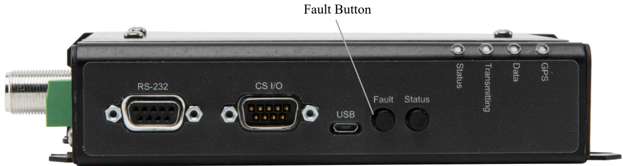
FIGURE 8-1. TX321 Fault Button
