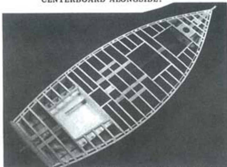
FRAMING AND BLOCKING OF DECK COMPLETE. CABIN TRUNK SOLE AND BUNKS FITTED AND PAINTED WHITE; CARGO HOLD HAS BEEN PAINTED RED LEAD COLOR.
