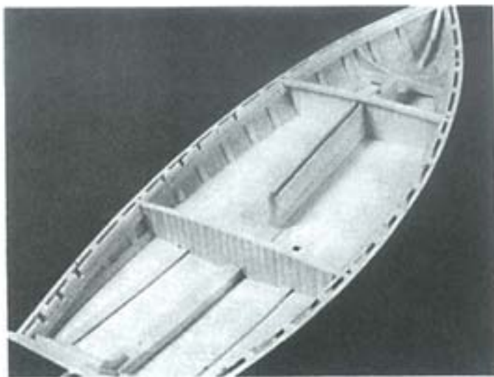
QUARTER VIEW SHOWING AFT SIDES OF HOLD BULKHEADS.
