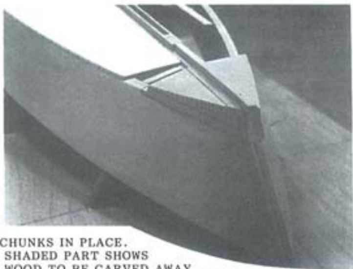
SIDE PLANKING IN PLACE WITH BOTTOM EDGE TRIMMED FAIR WITH CHINE. TOP EDGE HAS NOT BEEN TRIMMED TO FINAL SHEER PROFILE.
