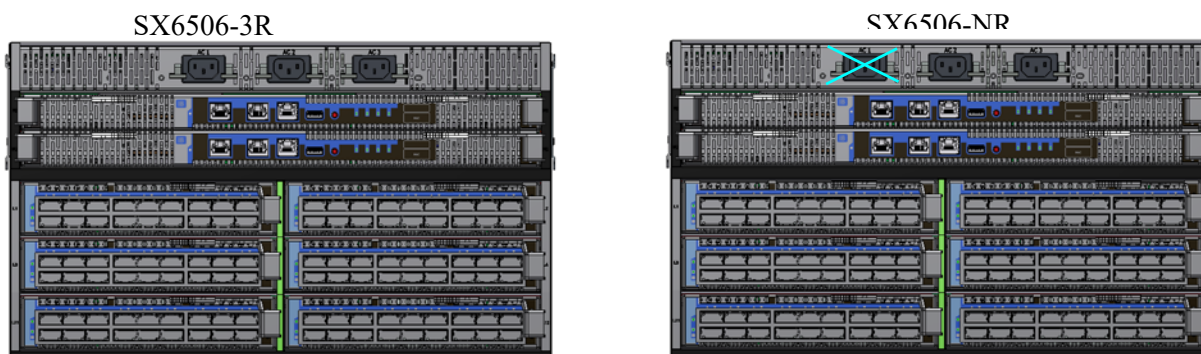
Figure 26: Do Not Use AC Power Socket #1 with N+N PSUs
