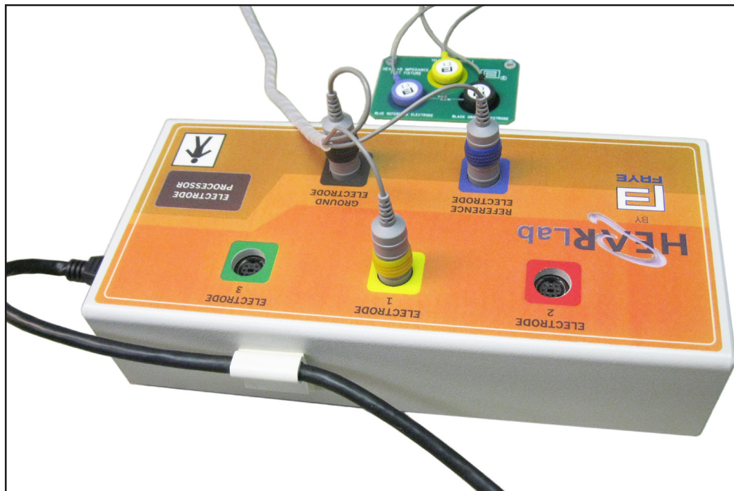
Figure 2.3.2: The electrode processor is connected to the stimulus controller through a special “firewire” cable.
