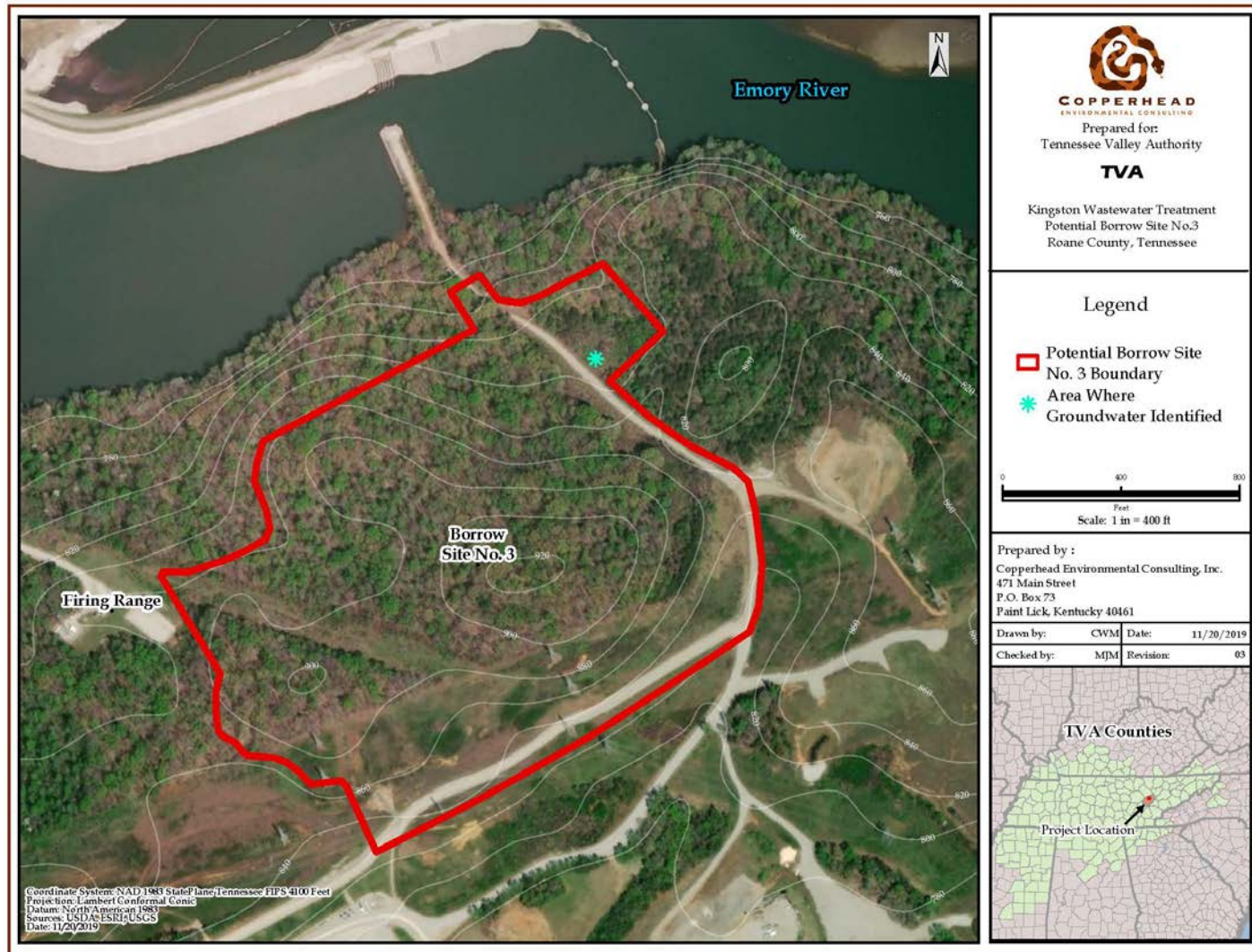
Figure 3-2. Groundwater Area Identified During Geotechnical Studies
