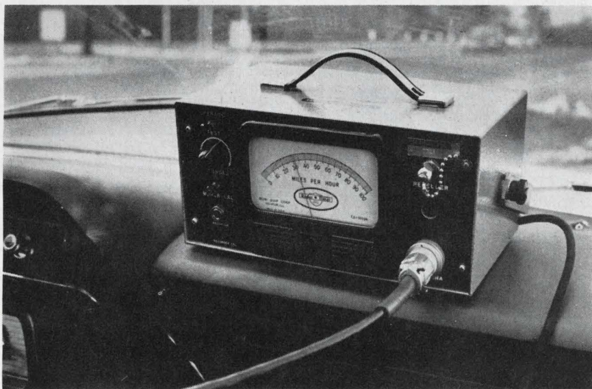
Pull over. Varian's Bomac division has developed an impatt diode as the microwave power source for police radar traps. Solid state device shrinks system into two packages—meter and controls, on the left, and antenna, right. But its price—still a few hundred dollars more than conventional gear—is keeping it out of the market. One design is being tested by the Mini Quip Corp.
