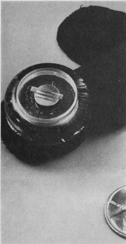
Guardian. Pulse of sleeping infant is monitored to prevent "crib death." Band fits on infant's arm.
