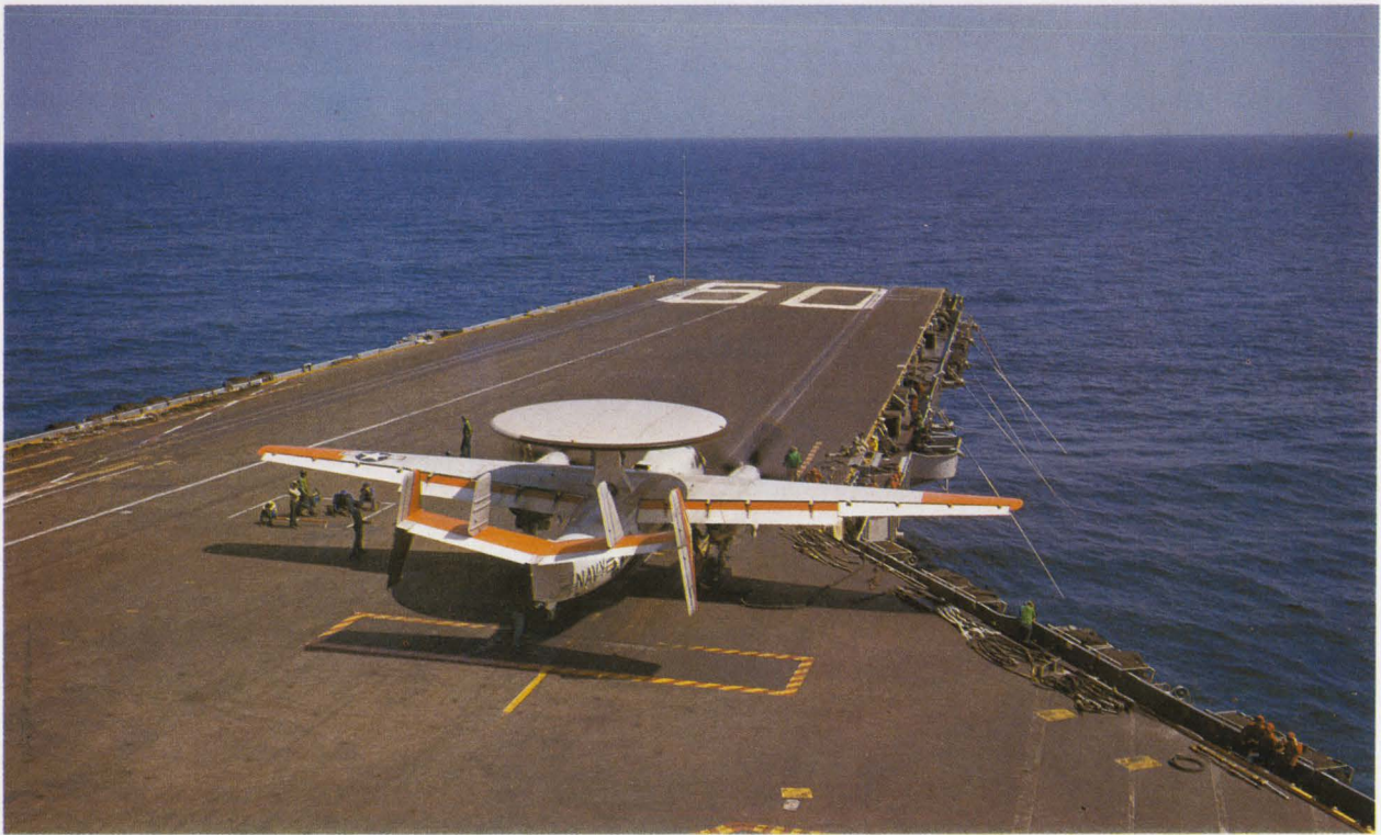
For openers. First extensive in-flight performance monitoring in an operational aircraft was developed by Grumman for the five-place E-2A Hawkeye used for early warning, command, and control.
