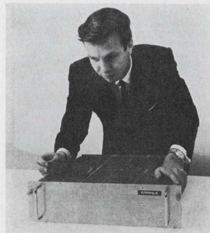
Three wires for speed. New 3-D memory fits in 19-inch rack.
