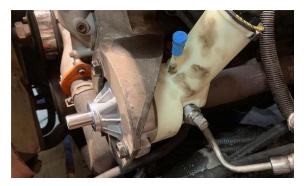
10. Install the PS pump and high pressure line.
