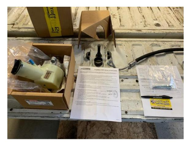
PS pump, pulley tool, and high pressure line. - Thank you Riffraff Diesel!! -
