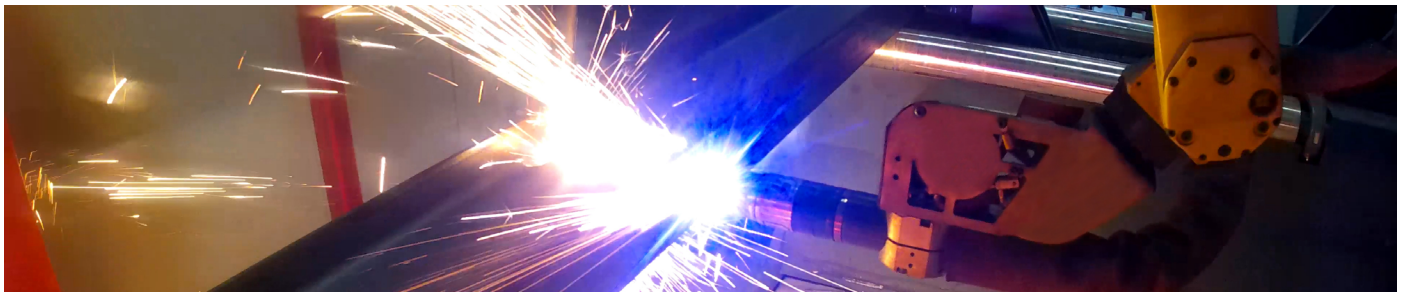
The plasma cutter cuts, copes, notches and splits beams much faster than traditional methods, reducing labor timelines and allowing more projects to be processed through AZCO's prefabrication and modular construction shop.
