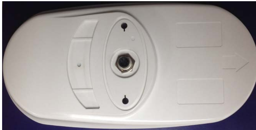
Figure 2-8: Flush mounting with holes in the V104n
