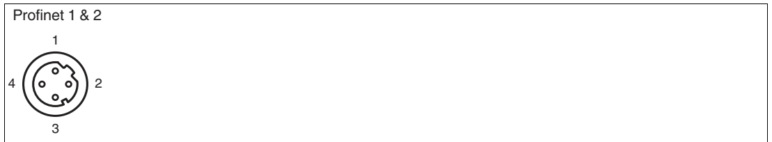
Figure 6.14 PROFINET connector assignment
