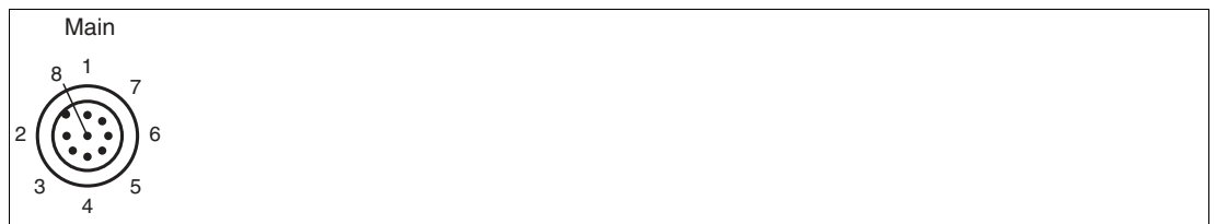
Figure 6.12 Connector assignment of the reader
