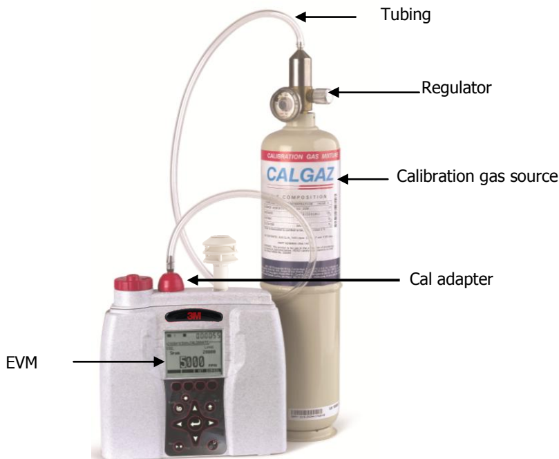
Figure 4-17: Applying a gas sensor
