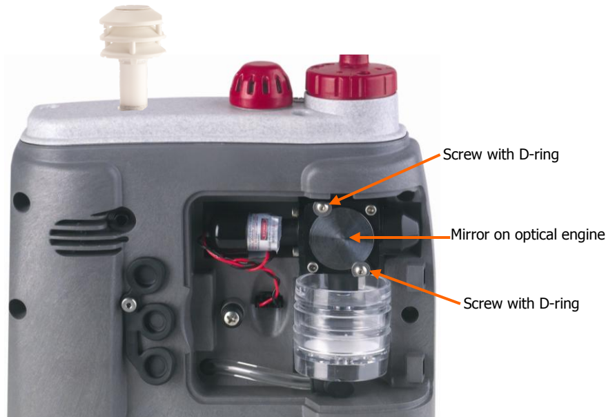
Figure 7-7: Optical engine and cleaning
