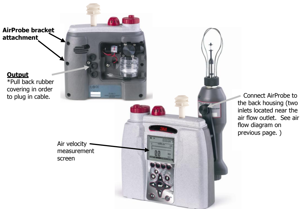
Figure 5-11: Attaching AirProbe and measuring Air velocity
