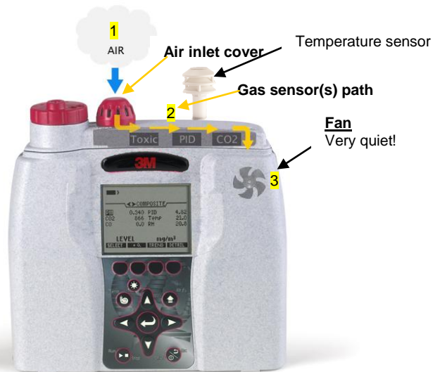
Figure 1-3: Gas sensor path illustration
