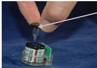
Figure 7-6: Fitting/Inserting the lamp and pellet
