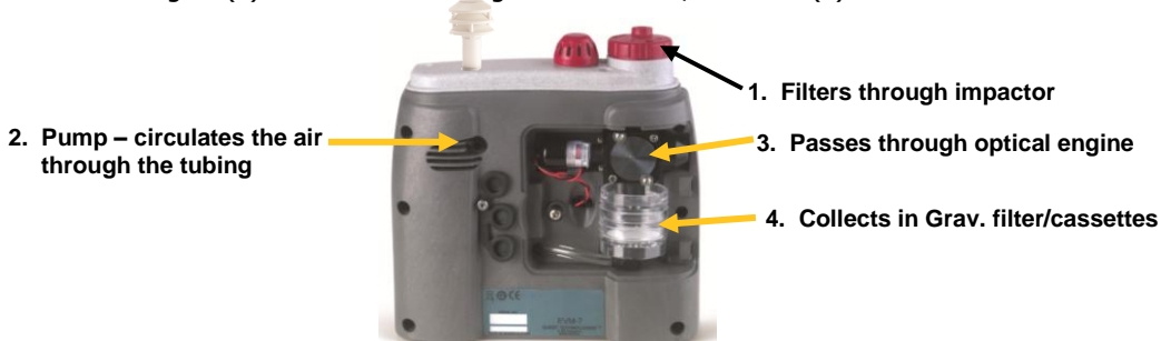
Figure 4-3: How the impactor functions
