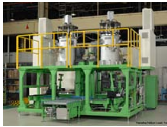
Helium leak tester
