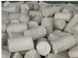
Sawdust pellets made from sawdust generated from the manufacturing of pianos
