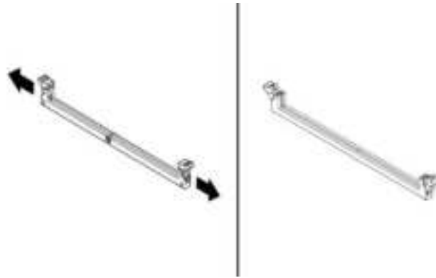
Figure 126. Opening the retaining clips
