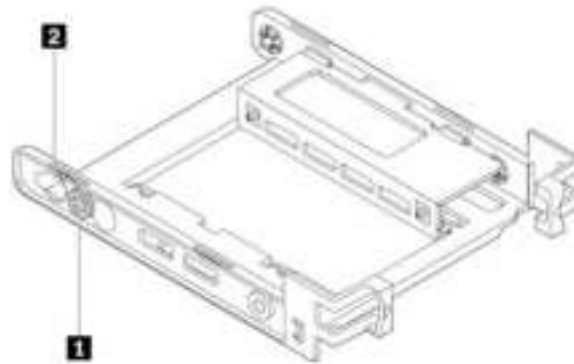
Figure 62. Removing the pin and installing it into the new slot
