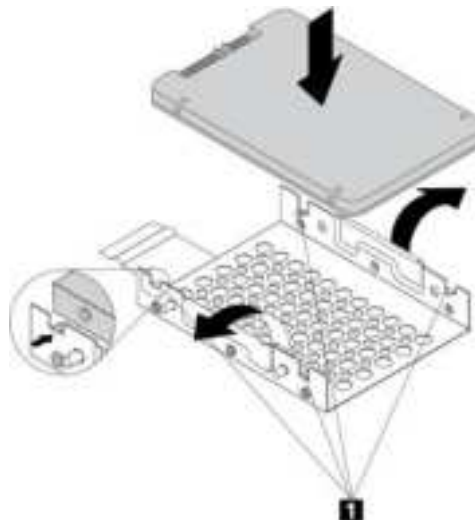
Figure 29. Installing the 2.5-inch storage drive into the metal bracket
