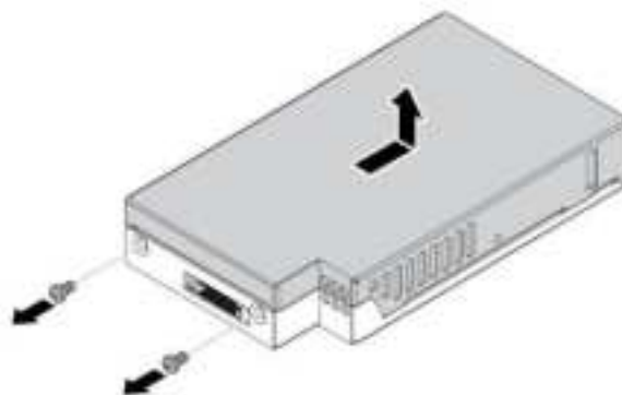
Figure 82. Removing the cover of the M.2 solid-state drive carrier
