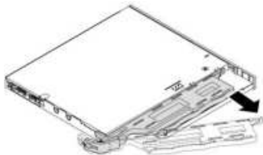
Figure 35. Removing the bracket from the slim optical drive
