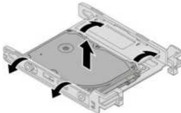
Figure 50. Removing the 2.5-inch storage drive from the bracket
