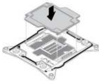
Figure 181. Installing the microprocessor socket cover
