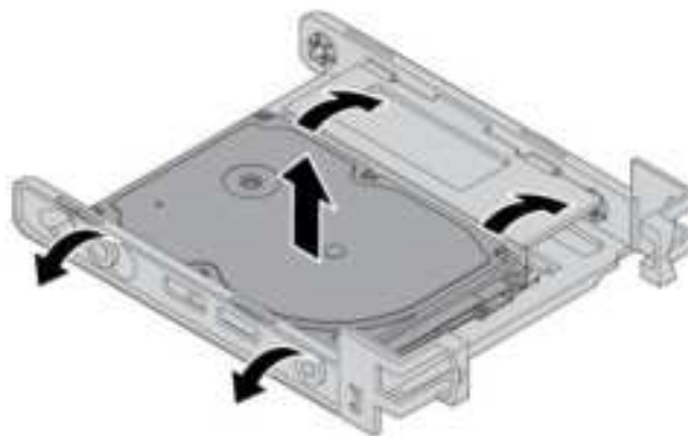
Figure 69. Removing the storage drive from the conversion bracket
