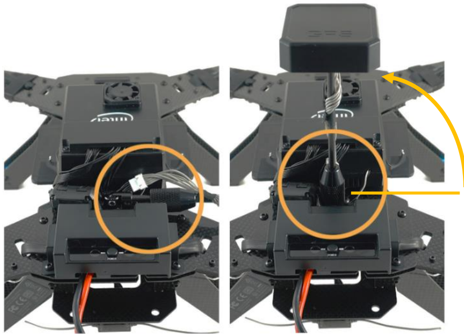
Figure 2. Raising the GPS Antenna Mast
