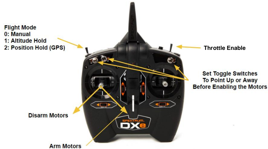
Figure 7. Transmitter Controls for Arming and Disarm the Drone Motors
