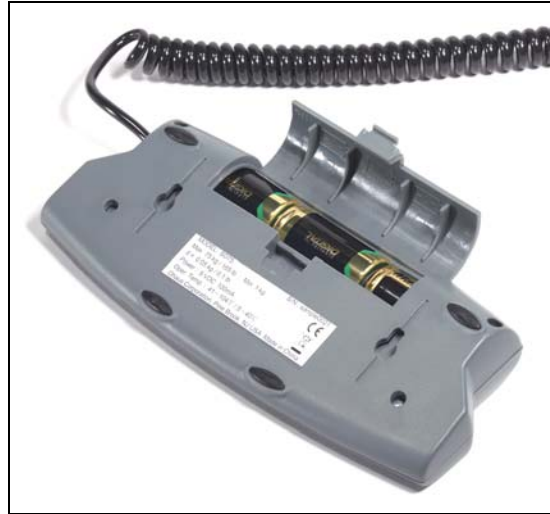
Figure 3-2. Open Battery Compartment door by pressing the inset latch lever.
