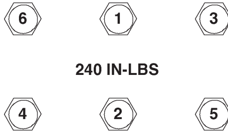
FIGURE 3. CYLINDER HEAD TORQUE SEQUENCE
