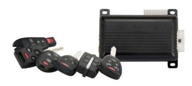
The ASP233ST will accept up to 4 remote transmitters, comes with a glass mount antenna with built-in LED lights and valet switch. It has a dual stage shock sensor (lite touch – full touch), starter interrupt output with relay included, onboard relay for flashing lights and start confirmation with parking light flash. The factory keyless upgrade input allows the factory
