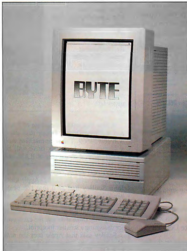
Photo 1: The Mac IIcx shown with the Apple Portrait Display. The reduced footprint covers an area of slightly more than a square foot. You can place the computer itself either horizontally or vertically.
