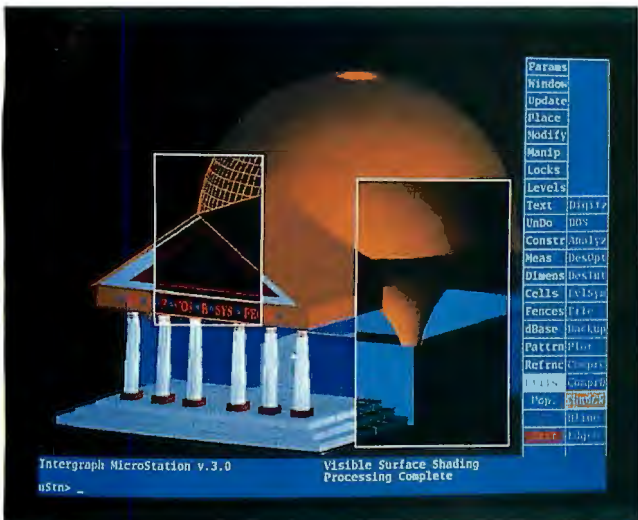
Photo 4: A MicroStation PC image on an Intergraph 19-inch monitor with a Matrox board.
