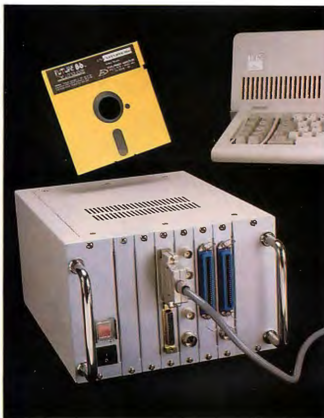
The UDM controls RS-232C and IEEE-488 I/O.
