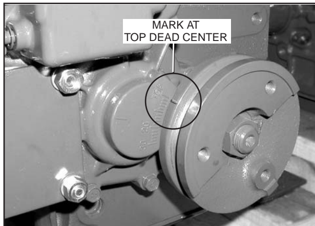
Figure 7-21. – Flywheel Position for Top Dead Center
