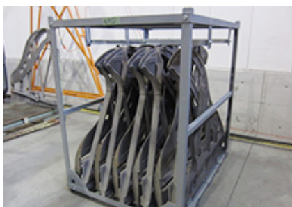
Returnable packing rack for grand piano frames
