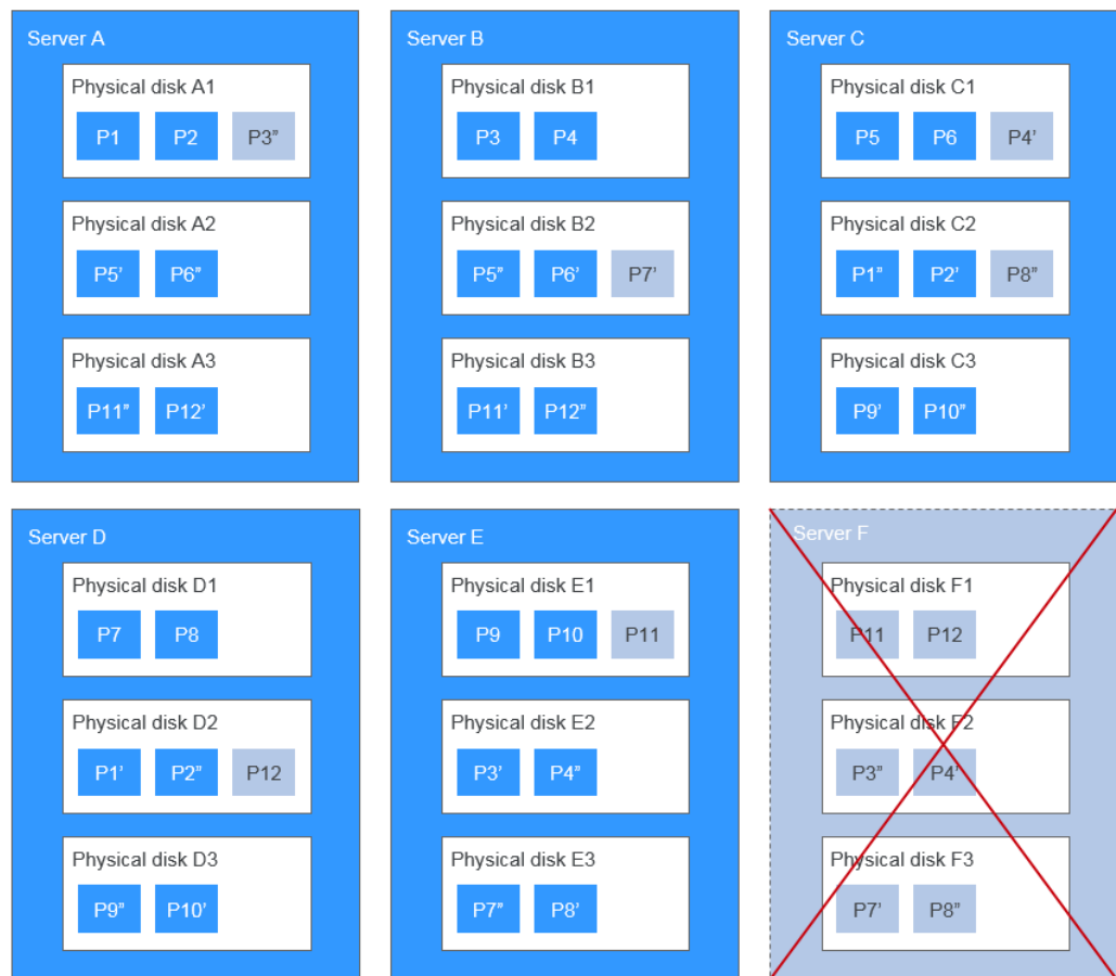
Figure 9-3 Data rebuild principle
