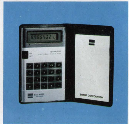
Solar cells keep the batteries continuously charged in these calculators by Royal Typewriter (top) and by Sharp (bottom). These units have liquid-crystal displays and CMOS.
