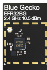
Figure 2.3. SoC Radio Board
