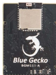
Figure 2.2. Module Radio Board
