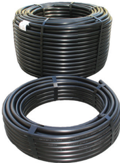
This polyethylene tubing is not rated for constant pressure. Use Easy Loc, or barbed fittings (p. 9, 10, and 24). Handles up to 50 PSI.
