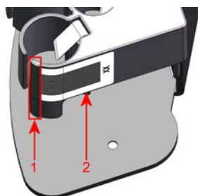
Figure 11. Aligning a barcode on the rack
