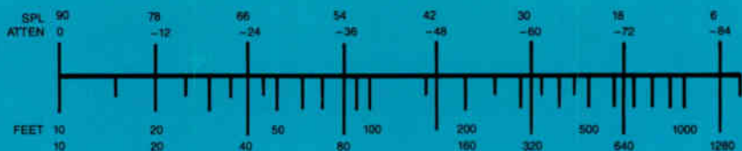
Fig. 1: The effects of outdoor distance on sound-level attenuation and background spl, for a 90dB source. The figures are approximate, depending on topology and ground cover.
