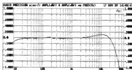
Fig.1 Carver Silver Seven-t, frequency response at 1W into 8 ohms (0.2dB/div.)
