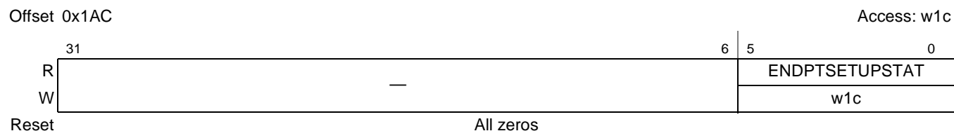
Figure 20-23 Endpoint Setup Status (ENDPTSETUPSTAT)
