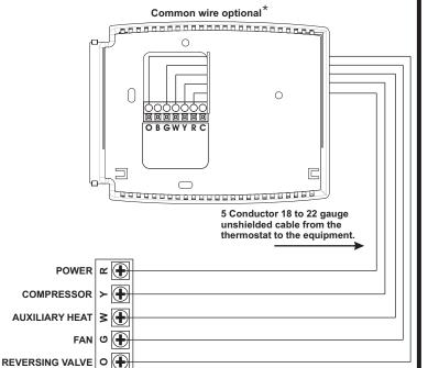
\* Common wire is optional in all installations. If a common wire is not used the thermostat must be powered by two AA alkaline batteries. These batteries must be replaced (page 11) each year or when the Low Battery indicator is displayed (page 3).
