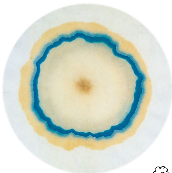
A reaction on filter paper: Berlin blue ring
