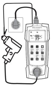
The preset value of the test voltage for the R<sub>ISO</sub> measurement is 500V. This voltage can be reduced to 250 V DC with the button (5), if needed. The selected test voltage appears briefly on the display then. By pressing the button (5) again, test voltage will be set back to 500 V DC.
