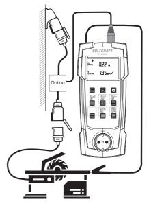
• The measurement is stopped if a contact voltage is present on the metal part of the test object. The warning can be seen on picture on right side.
